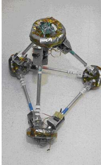
Fig. 1. NASA TETwalker prototype assembly that will provide the rough model prototype http://t2www.nasa.r3h.net/images/content/111408main_tetwalker_4.jpg
